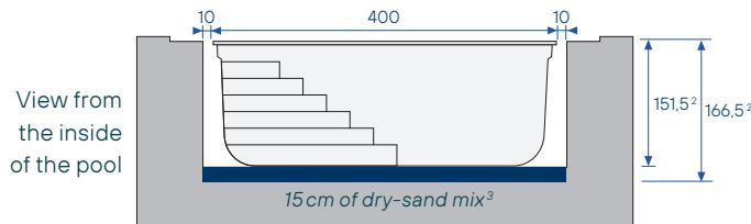
Note: the digging sizes do not take into account the necessary space for the coping stones.
