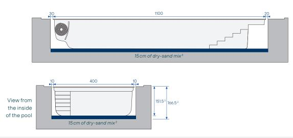
Note: the digging sizes do not take into account the necessary space for the coping stones. <sup>1</sup> Needed for unloading & placing the pool. <sup>2</sup> Depth taken from under the coping stone. <sup>3</sup> Mix of sand and cement, at a ratio of 250 kg per ton.
